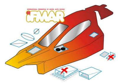
If no "marked" air scoops/vents are designed in the original mould to assist airflow to the motor or ESC, then material may be removed to a maximum of 10 mm in any given direction within a maximum square area of size 30 mm x 30 mm, in two places only. Windows are not allowed to be removed or include holes, other than for the purpose of the antenna.
